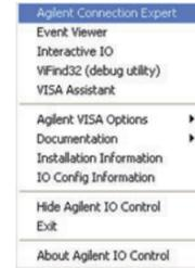
3. Select the PC's GPIB interface and select 'Add Instrument' from the Connection Expert menu bar.
